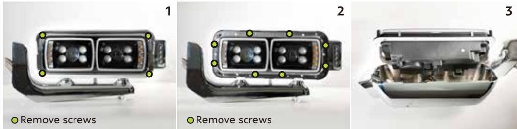
1. Remove headlight bezel by removing the 4 screws.
