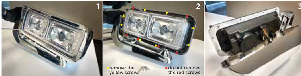
1. Remove headlight bezel by removing the 4 screws.
