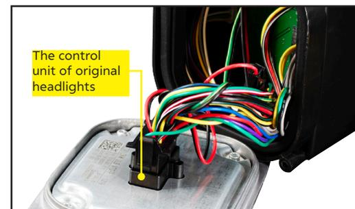
**Step 3:** Connect the plug of new headlights with the control unit of original headlights.
