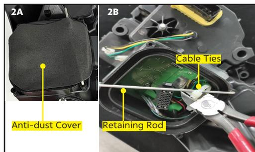
**Step 2A:** Please remove the anti-dust cover on the back of new headlights.
