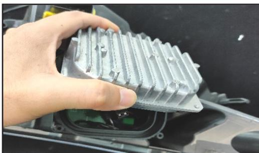
**Step 4:** Assemble the control unit of original headlights with the new headlights.
