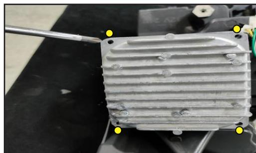
**Step 5:** Tighten the 4 screws to fix the control unit on the new headlights.
