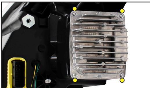
**Step 1:** Please remove the control unit from the original headlights by unscrew the 4 screws in control unit and preserve it.
