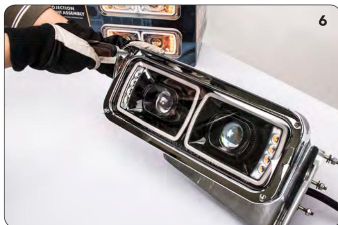
**Special Installation Note:** If fuse blows on high beam, please flip the high beam plug over 180 degrees.
