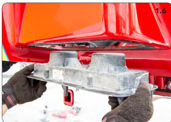
**2.** The new fender liner mounts under the fender from the back. Some trucks might have an extra support bracket that will need to be loosened enough to slip the new fender liner under the bracket. Drill and enlarge the holes as necessary for installation of the 4 screws. Mount the new fender liner in place with the screws and nuts. Install the headlight wiring through the center opening of the new fender liner.
