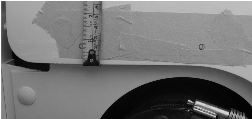
The two horizontal mounting holes should be marked on a shared horizontal centerline,  $\frac{3}{4}$ " from the edge of the hood above the intake boot as shown above.
