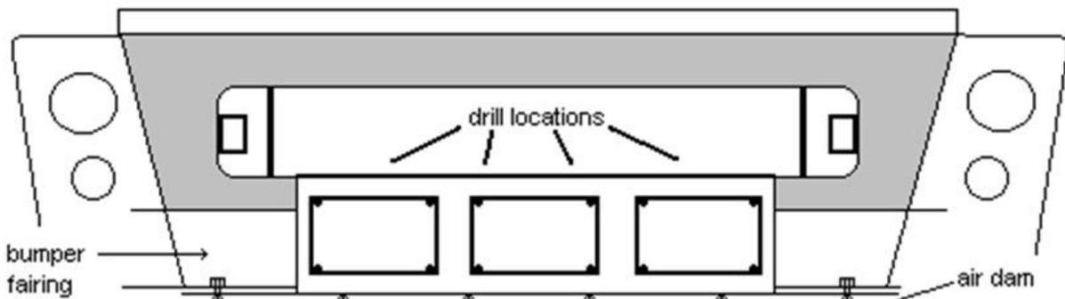
5. Drill 7/32" or 3/16" holes through holes in license plate holder into bumper. (if available, use an "Angle Drill")
