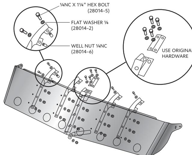
6. Fasten the sides of the sun visor to the cab with the original sunvisor hardware. Feed the screw and flat washer through each of the 4 holes. Tighten with the original well nuts.
