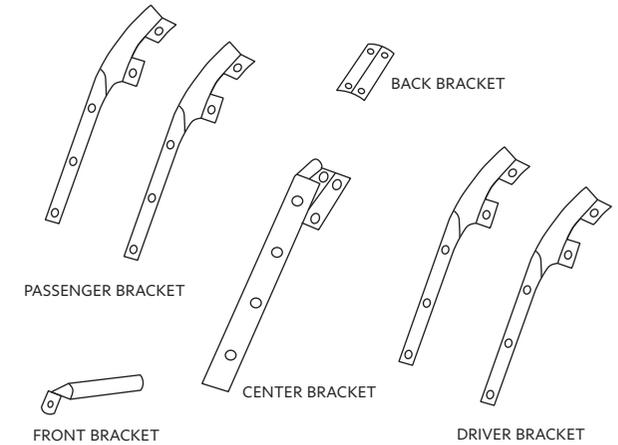
4. Fasten each screw to all brackets with a 1/4 lock washer and 1/4 hex nut on the back side of the bracket.
