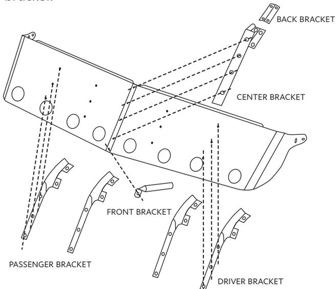
5. Attach the brackets to the cab with the 1/4NC x 1 1/4" hex bolt. Feed the 1/4NC x 1 1/4" hex bolt and a 1/4 flat washer through each hole of the bracket. Fasten the hex bolts with the 1/4NC well nut on the back.
