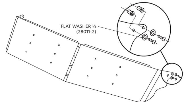
\* Depending on the year of the truck, holes may need to be drilled on the front of the cab for proper installation
