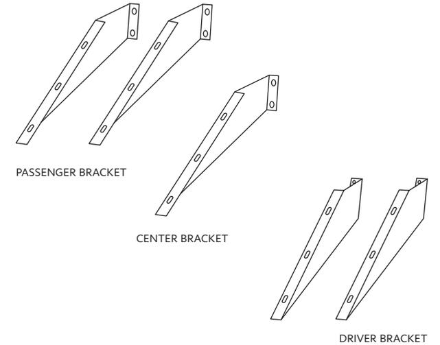
4. Fasten each screw to all brackets with a 1/4 lock washer and 1/4 hex nut on the back side of the bracket.
