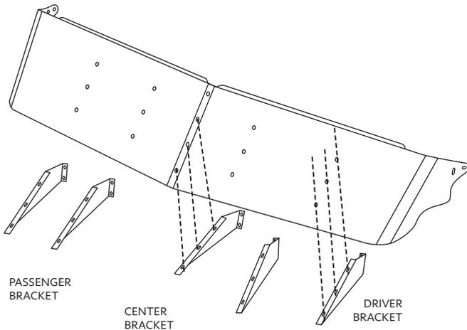
5. Attach the brackets to the cab with the 1/4NC x 1 1/4" hex bolt. Feed the 1/4NC x 1 1/4" hex bolt and a 1/4 flat washer through each hole of the bracket. Fasten the hex bolts with the 1/4NC well nut on the bracket.
