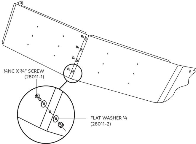
2. Feed the 1/4NC x 3/4" screw through the twelve remaining openings.
