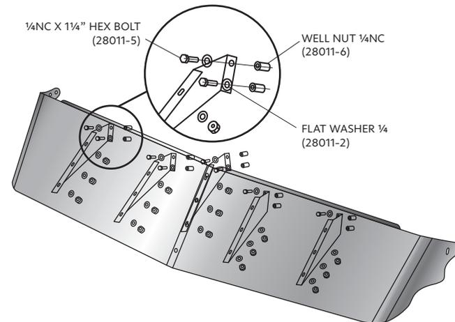
6. Fasten the sides of the sun visor to the cab with the original sunvisor hardware. Feed the original screw and 1/4 flat washer through each of the 4 holes with original well nuts.
