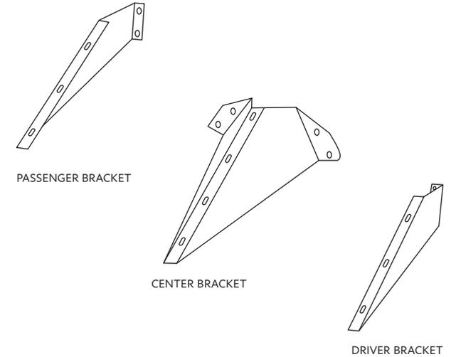
4. Fasten each screw to the bracket with a 1/4 flat washer and 1/4 hex nut on the back side of the bracket.
