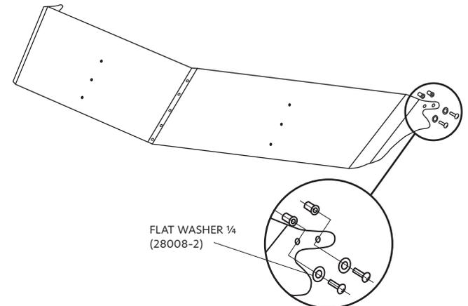
\* Depending on the year of the truck, holes may need to be drilled on the front of the cab for proper installation
